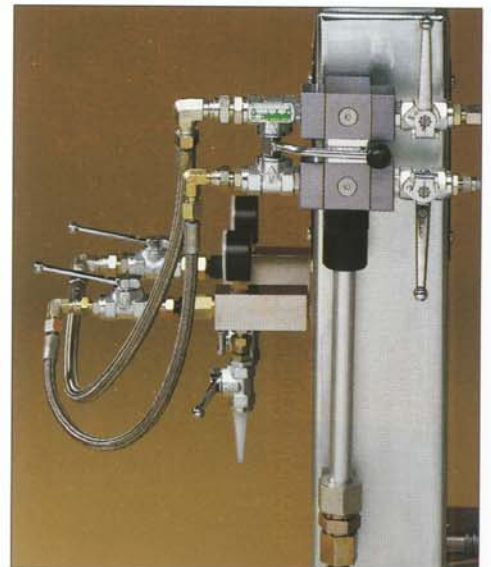
▲ Static mixer unit (mixing block with static mixer pipe)
