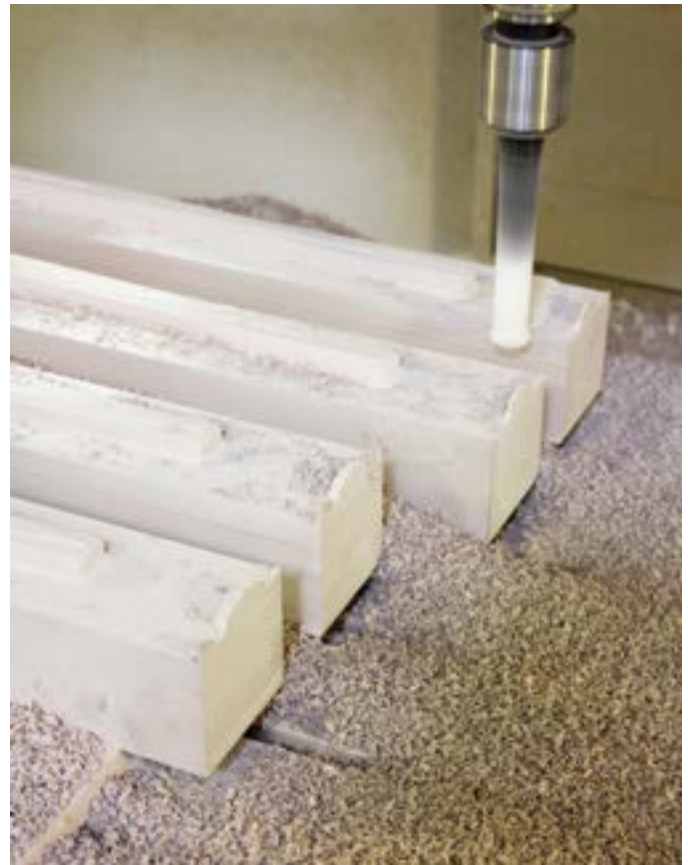
RenShape 460 offers an excellent surface finish for many large and lightweight styling applications.
