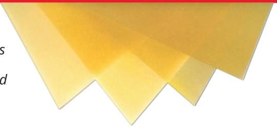
▶ **Freeman Sheet Wax** is used primarily to simulate metal or part thickness when making metal forming dies or punches, resin transfer molds (RTM), or any two-part molds requiring a uniform part thickness. Formulated and manufactured by Freeman, these waxes are available in most thicknesses from .007" to .394" with a tolerance of  $\pm .001$ ". Adhesive for these waxes can be applied manually with Freeman's Sheet Wax Adhesive Spray.
