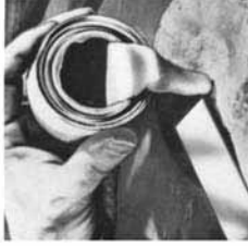
Lab-metal spreads like paste and hardens into metal. Application tip: wet the applicator with Lab-solvent to aid in smoothing the Lab-metal and reduce "pulling".
