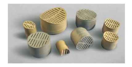
Ventistamp's curved and inclined vents have revolutionised the concept of tool ventilation, due to their slots that follow the geometry of the cavity while preserving the internal taper.
