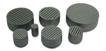
MeltVents-KT is a super self-cleaning vent line, which represents the concept of slotted vents. They are manufactured in Carbon Steel alloy, and feature slots with inverted taper. This is a vent line suitable for any volume production, in the Gravity and Low Pressure Aluminum processes.
