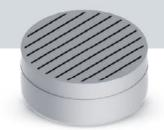
Slot of 0.4mm and inverted taper - Recommended only for the regions of the permanent mold where the vent gets into contact with the sand core, for low pressure and gravity processes
