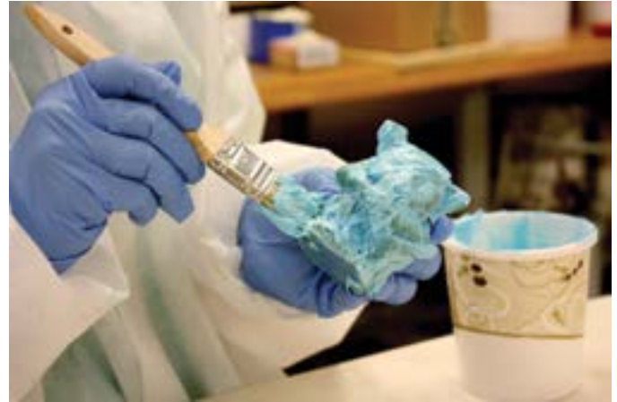
Thixo Additive can be added to V-340 to create a brushable silicone material, used here as a component of a glove mold.
