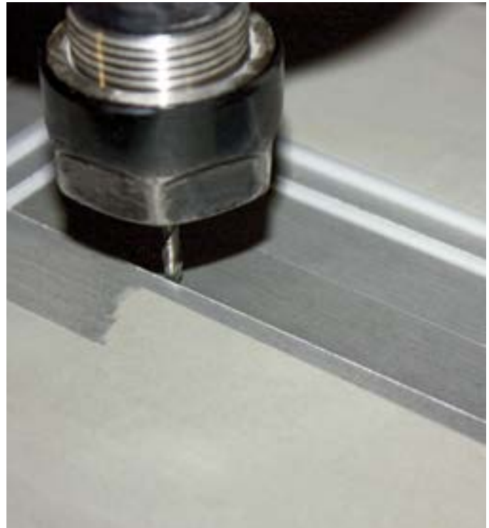
RenCast 4037 can be machined for an incredibly smooth surface finish.
