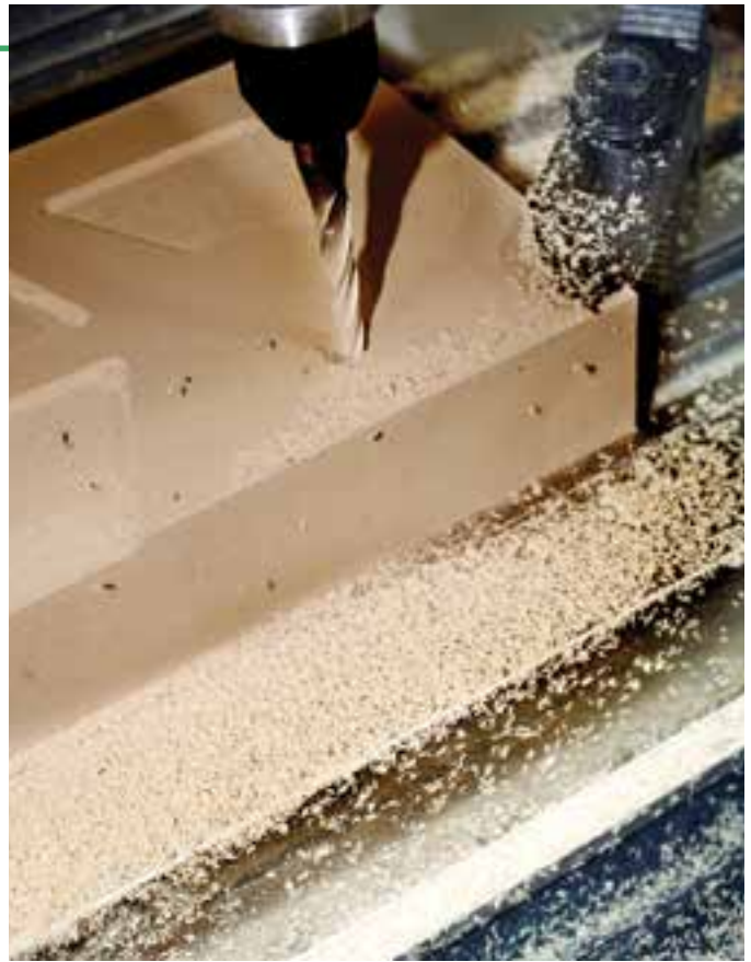
RenShape 5035 and RenShape 5045 (pictured) work extremely well on the CNC. They create flakes rather than dust when machined, allowing for fast, easy clean-up.
