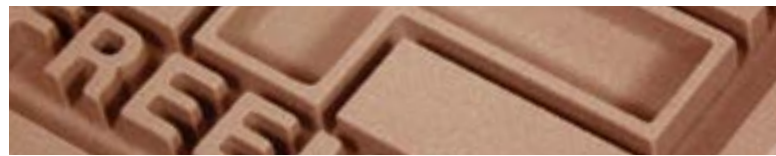
RenShape 5035 and RenShape 5045 (pictured) work extremely well on the CNC. They create flakes rather than dust when machined, allowing for fast, easy clean-up.
