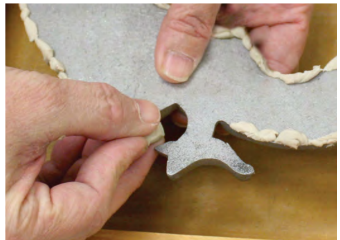
Clays can be used to adhere a part to the mold box.
