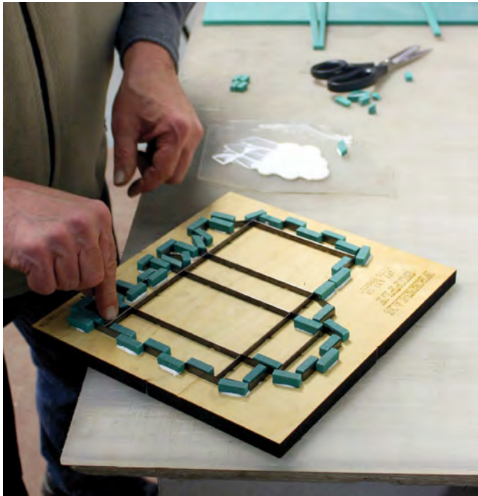
A diemaker uses DieStrip Adhesive to secure ejection rubber (page 110) next to the steel rule (page 109).
