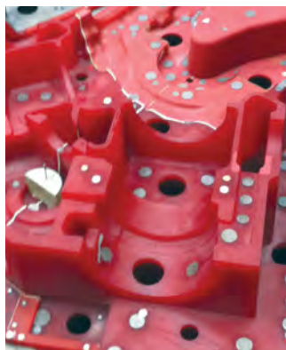
Vent Plugs are used to seal vent holes.
