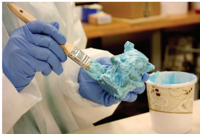
Thixo additive can be added to V-340 to create a brushable silicone material, used here as a component of a glove mold.
