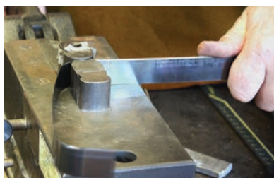
HS CITO Steel Rule and Freeman Ejection Rubber are used here on Freeman's UltraFlat Maple Dieboard to create a die for a reverse tuck box.
