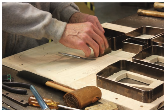
Our CITO Steel Rule (page 109) can be applied to a die board with a rawhide mallet. (page 110)
