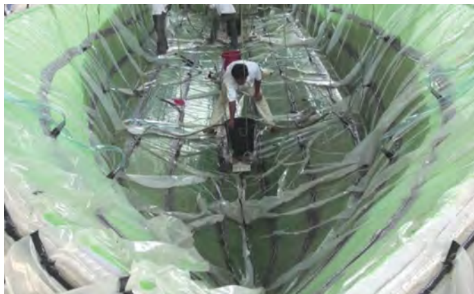
These systems are designed for the Seemans Composite Resin Injection Molding Process (SCRIMP SM ), used on boats and other nautical applications.
