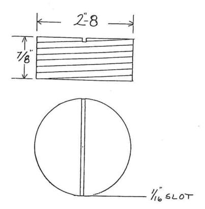
SQUEEZE BOARD STOP-OFF- SLOTTED (PART NO. 34022P)
