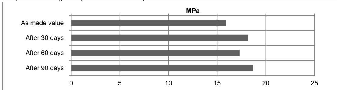
**Lap shear strength versus heat ageing at 70°C (ISO 4587; typical average values)**
