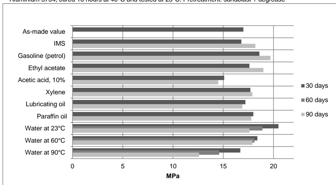
**Lap shear strength versus tropical weathering (DIN 50015; typical average values)**
