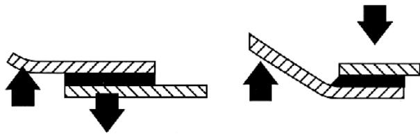
A peel joint can be designed such that the forces acting upon it become compression forces, making a much stronger joint.
