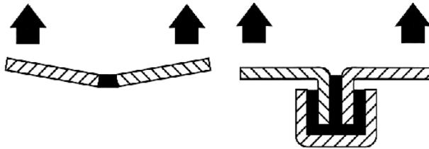
Weak cleavage joints can be strengthened through design, in this instance by adding a U-section to the previously bent sheet.
