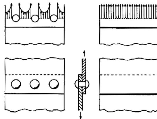
**Fig. 2 Stress distribution in loaded joints**
