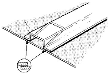
**Fig.8 Stiffening of large thin sheets**
