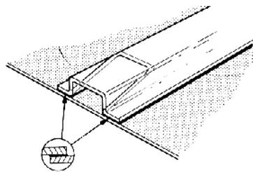
**Fig.8 Stiffening of large thin sheets**
