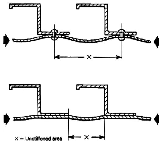
**Fig.1 Stiffening effect – bonding and riveting compared**
