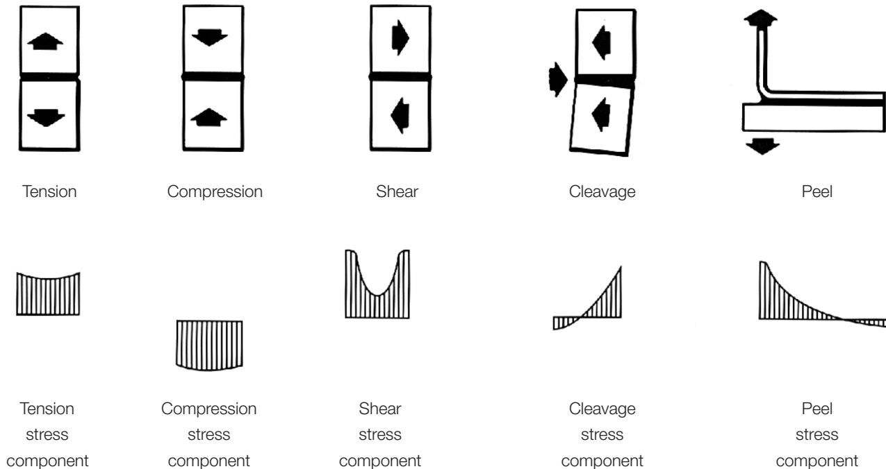
**Fig.1 Loading conditions**
