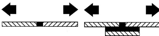
By adding reinforcing plates to this butt joint, the forces run along a much stronger shear joint.
