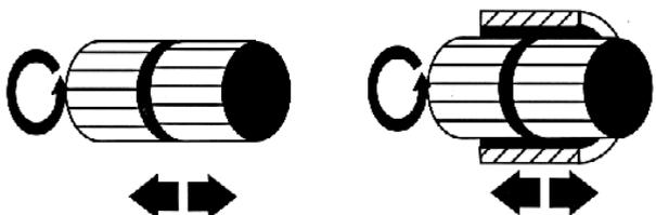
A similar effect is produced by sleeving this cylindrical butt joint.
