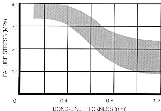
**Fig.10 Bond-line thickness vs. shear strength**
