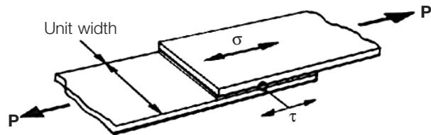
**Fig.14 Conventional designs for stresses in a lap joint**
