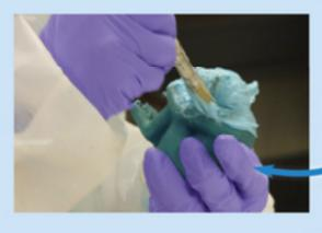
Using the glove mold technique, even complicated parts can be easily reproduced! Here, our Tech Team uses Bluestar Silicone V-330 with the CA-35 catalyst. This silicone combination offers both high tear strength and high elongation properties, perfect for creating a flexible glove mold. A third component, Bluestar Thixo Additive, is added to increase the viscosity of the silicone from pourable to brushable. Here's how they did it:
