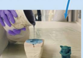
3. With the original part removed and mold secure, cast a new part. <u>Repro Fast-Cast Urethanes</u> are a popular choice for quick casting and demolding!
