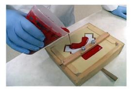
Casting Thin-Walled Parts
