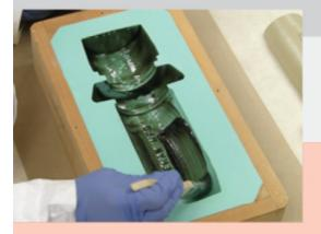
For tools with intricate details, this technique is more ideal than surface casting. Freeman 1060, when used as a durable surface coat, will easily replicate details such as lettering and texture with no air entrapment.
